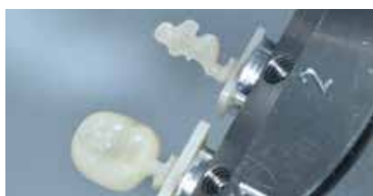
Restoration after completion of milling
