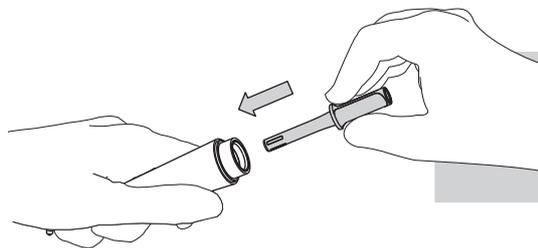
Clean the handpiece with the EasyClean supplied with the unit before disinfecting and sterilizing.
