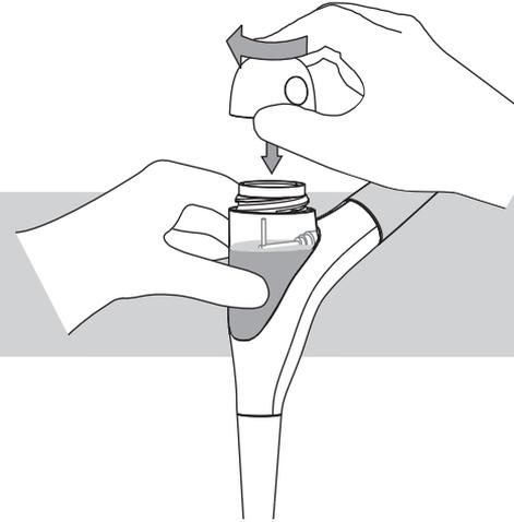
Clean the threads of the powder chamber before screwing on the cap.
