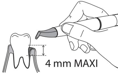
Direct the nozzle strictly towards the surface of the tooth. Respect a distance of 3 to 5 mm.
