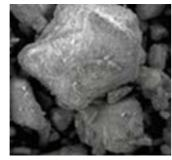
Particles with softened geometry (x1000)
