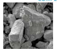
Stratified particles with aggressive geometry (x1000)
