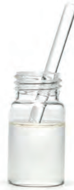
The refractive index of the monomer matrix matches that of the fillers - in this case, of the glass rod. It appears nearly invisible.
