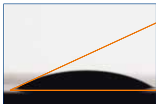
Impregum Garant L Duo Soft – contact angle of ~ 24°
