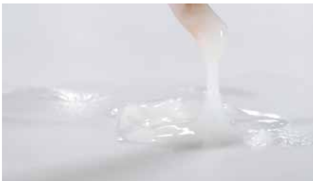
If mixed correctly the consistency of the glazing material must not be too liquid.
