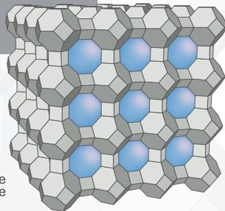
Nanoporous structure of Silver Zeolite
